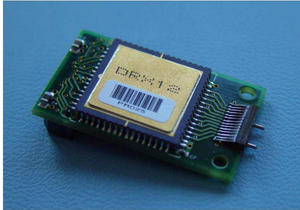
Figure 3.23.: RX plug-in with a size of 1.5 cm \times 3.5 cm, which transforms the received optical signals into electrical and passes them to the BOC [12].
