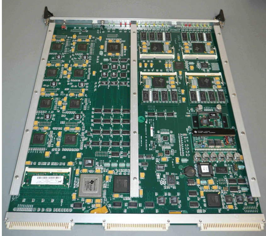
Figure 3.28.: The Read Out Driver (ROD) as it is used for SCT and pixel detector.
