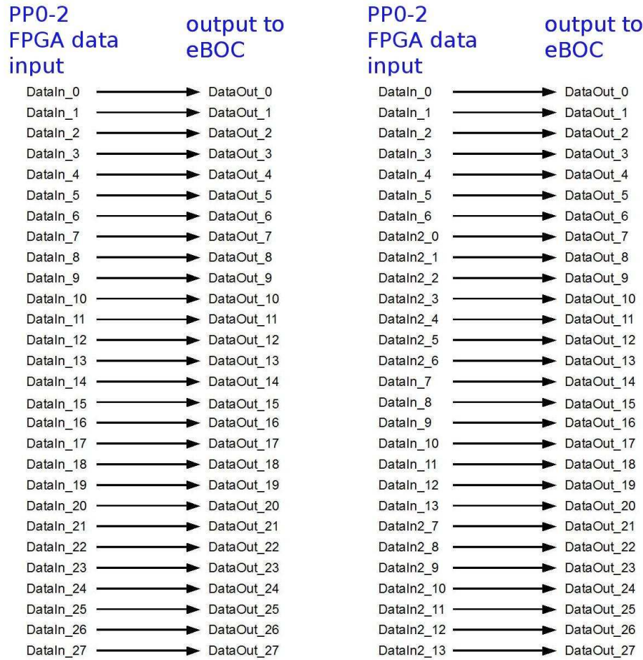
Figure 5.4.: PP0-2 FPGA data routing, left for 1 \times 40 MBit/s and 1 \times 80 MBit/s mode and right for 2 \times 40 MBit/s and 2 \times 80 MBit/s mode.
