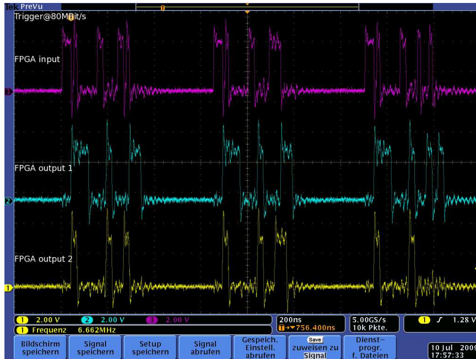
Figure 5.8.: Trigger-response sent by the module to the eBOC at 80 MBit/s. The colour code of the lines is the same as above, but the length of one bit at the FPGA input line is 12.5 ns, at the two FPGA outputs it is 25 ns.
